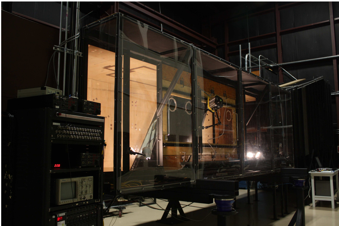
Figure 2.6: SWIFTEST in the KSWT with IR camera installed in middle port
