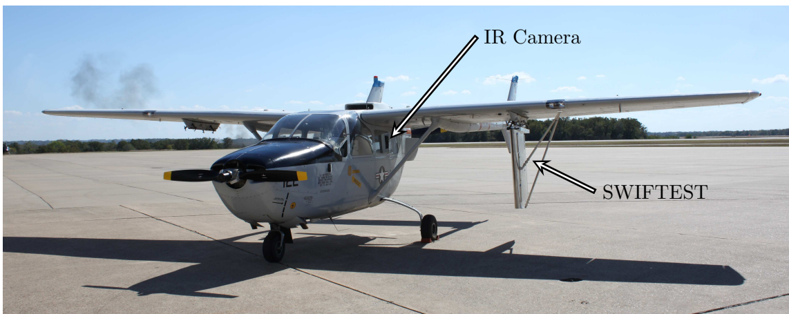
Figure 2.5: SWIFTEST installed on a Cessna O-2A Skymaster
