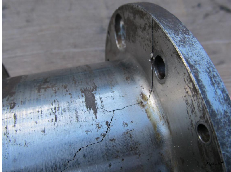
Fig. 23 Broken coupling hub
