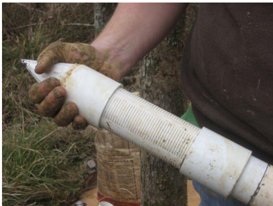
Figure 3. Picture of the well screen attached to the bottom of the well body
