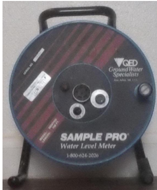
Figure 5. The Sample Pro Water Level Meter used to monitor the wells at ABNC
