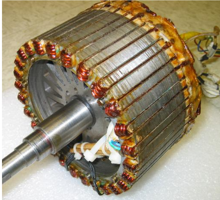
Figure 24 Photograph of the prototype single layer FSCW stator with 54 slots and 4 conductors per slot
