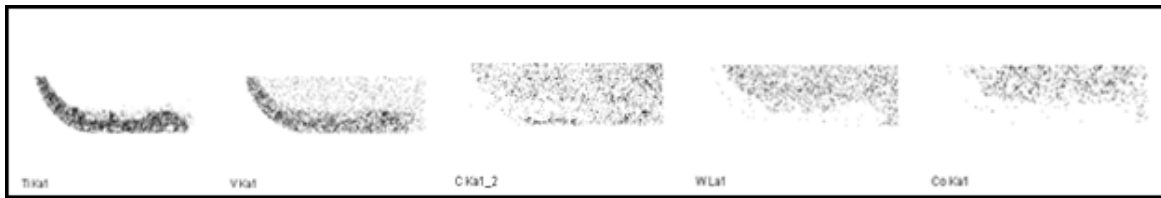
Figure 4-7 EDS images of composition of elements in cutting tool when cutting speed is 60m/min and feed rate is 0.15 mm/rev after machining 10 cm 3 . The elements are Ti, V, C, W, and Co from left to right.
