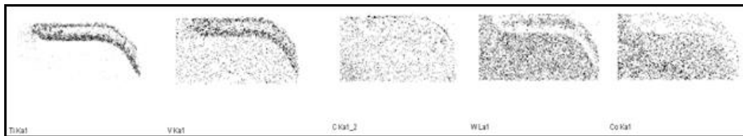
Figure 4-28 EDS image of composition of element in cutting tool when cutting speed is 120m/min and feed rate is 0.15 mm/rev after machining 30 cm 3 . The elements are Ti, V, C, W, and Co from left to right.
