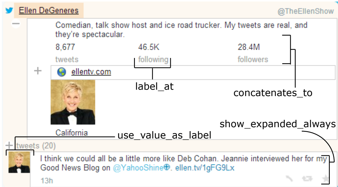
Figure 5.4: Presentation semantics enable highly detailed metadata expansion. The rendering of Ellen’s @username feed is customized with semantics concatenates_to , navigates_to , hide_label , and label_at (See Tables 5.1 and 5.2). The twitter_microblog metadata type plays a central role (See Figure 5.3).
