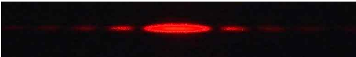
Fig. 2. Photograph of the interference pattern resulting from a laser beam going through a single slit [12].
