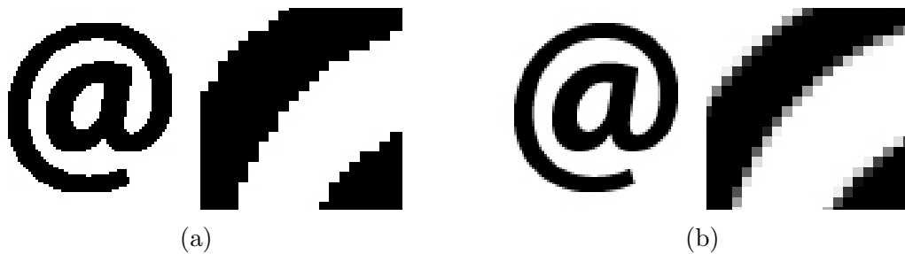
Figure 4.3: Examples of anti-aliasing. (a) is a large atmark rendered without anti-aliasing. (b) is a large atmark rendered with antialiasing. Antialiasing smoothes out the jaggies.
