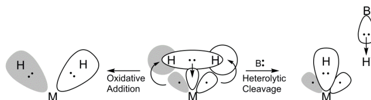
Figure I-3. H 2 binding with H 2 \sigma -donation and \pi -back donation into H 2 \sigma^* (center), the oxidative addition of H 2 , forming a M n+2 (H) 2 complex (left), and heterolytic cleavage leading to deprotonation (right). 36,41
