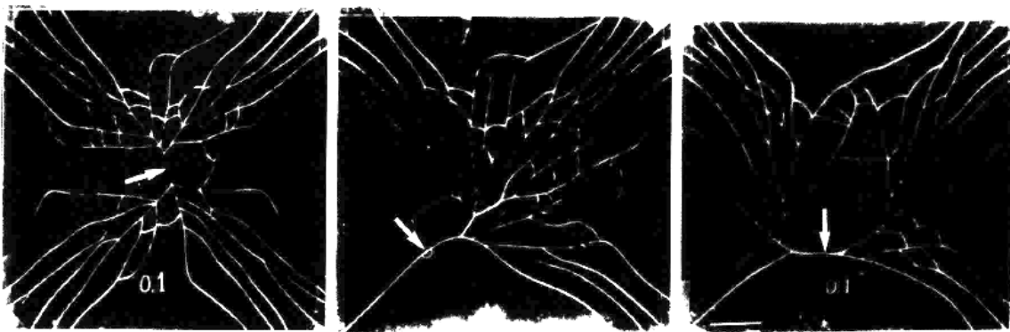
Figure 23: Crack Patterns Produced on Flat Glass from Uniform Loading [35] (Arrows indicate the initiating points of the fractures)
