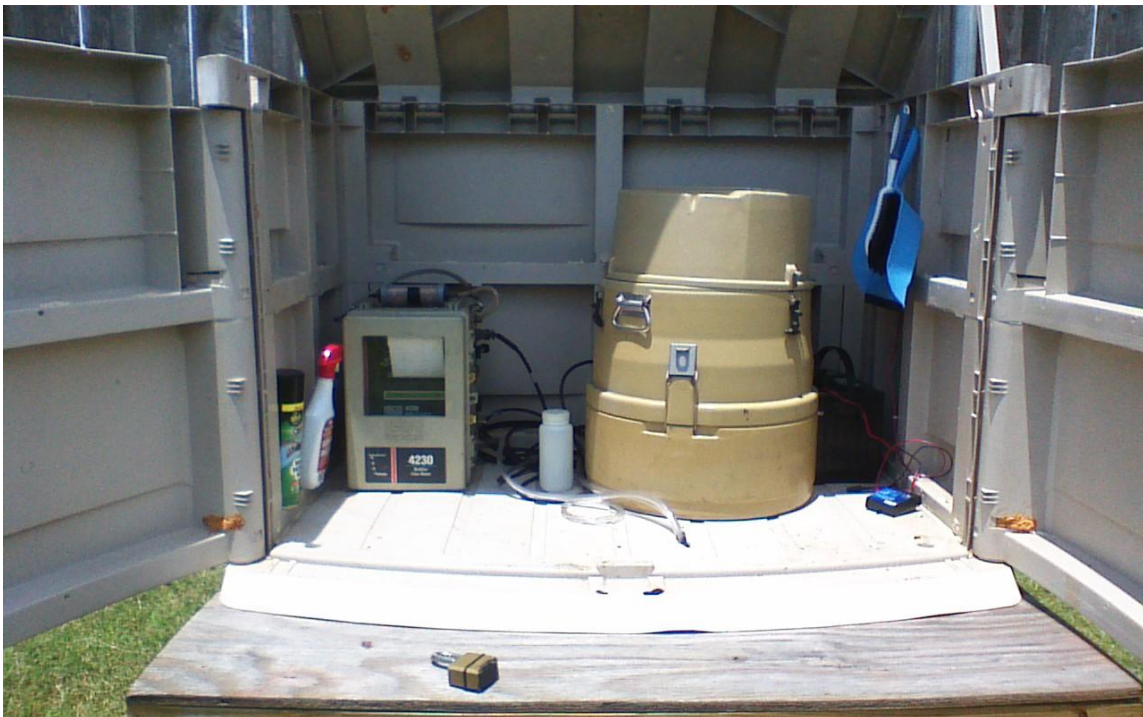
Figure 9. Bubbler flow meter (left) and automatic water sampler (right) used to collect runoff at the control site.
