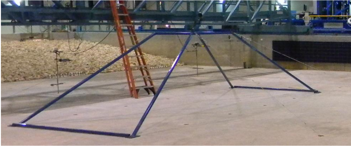
Figure 52. Support frame with guide wires, without breakwater
