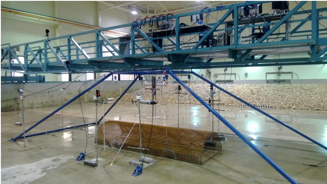
Figure 13. Submerged breakwater with instrumentation and DAQ system on bridge.
