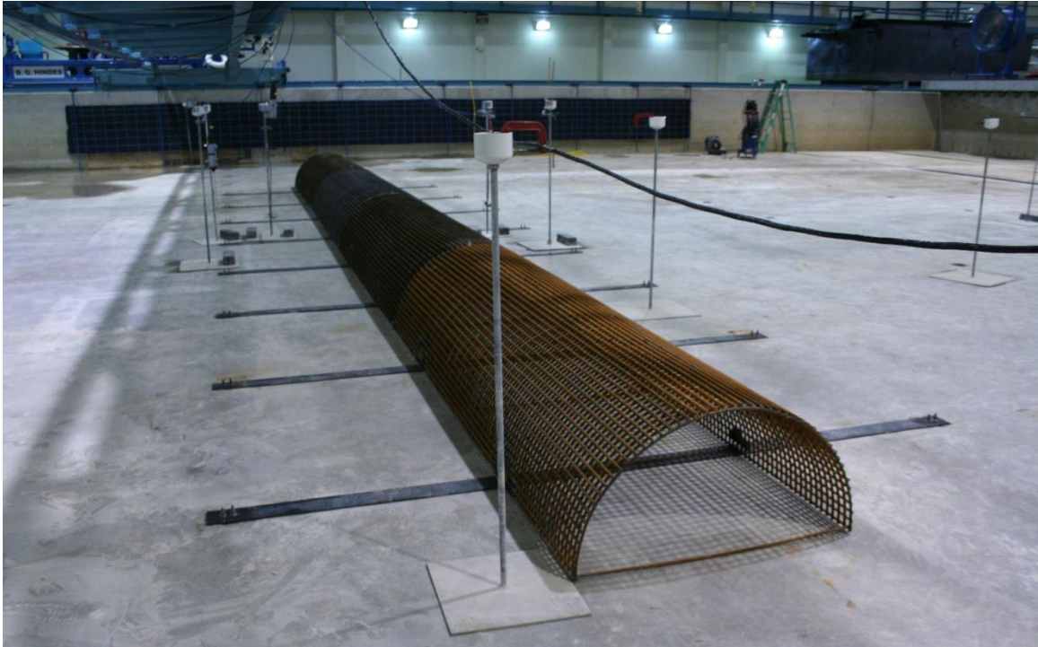
Figure 62. 40 ft breakwater wave transmission reflection setup
