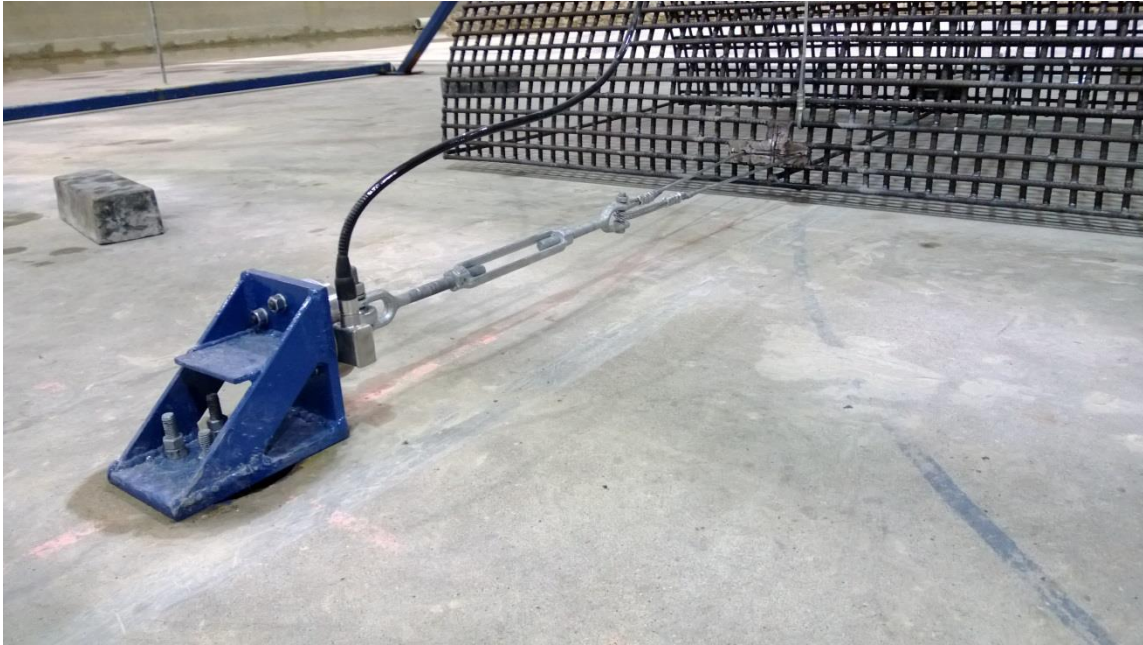
Figure 57. Front horizontal force reaction cable with force gauge and support
