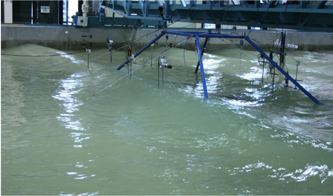
Figure 61. During force testing of breakwater
