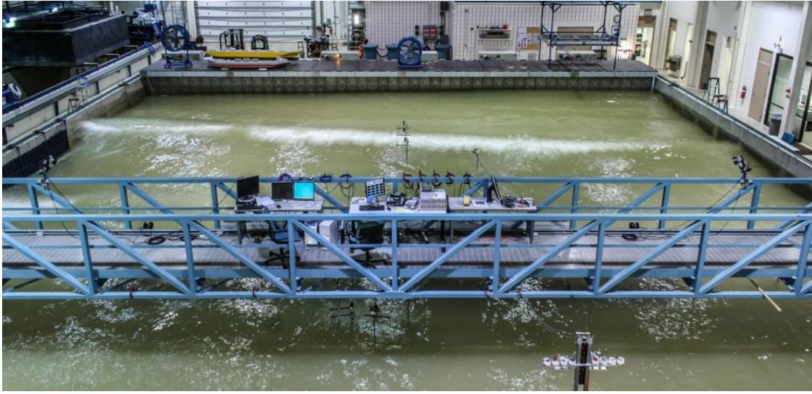
Figure 4. Shallow water wave basin in the Haynes Coastal Engineering Laboratory.
