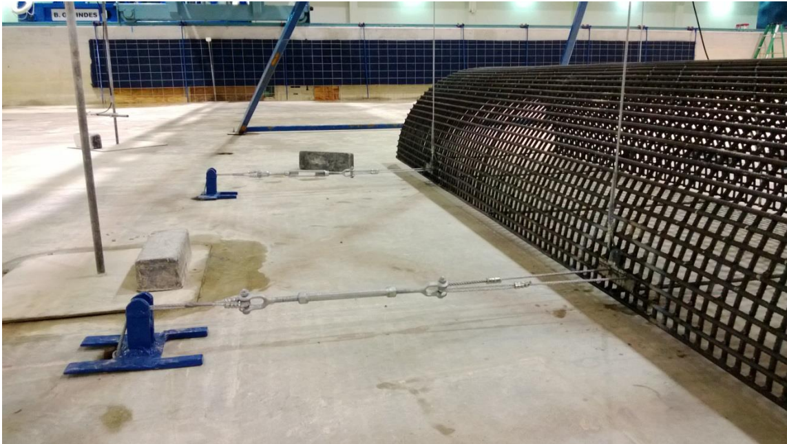
Figure 56. Rear horizontal force reaction cables with supports
