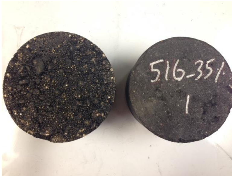
Figure 20. EPP modified asphalt concrete (left) and graphite modified asphalt concrete (right)
