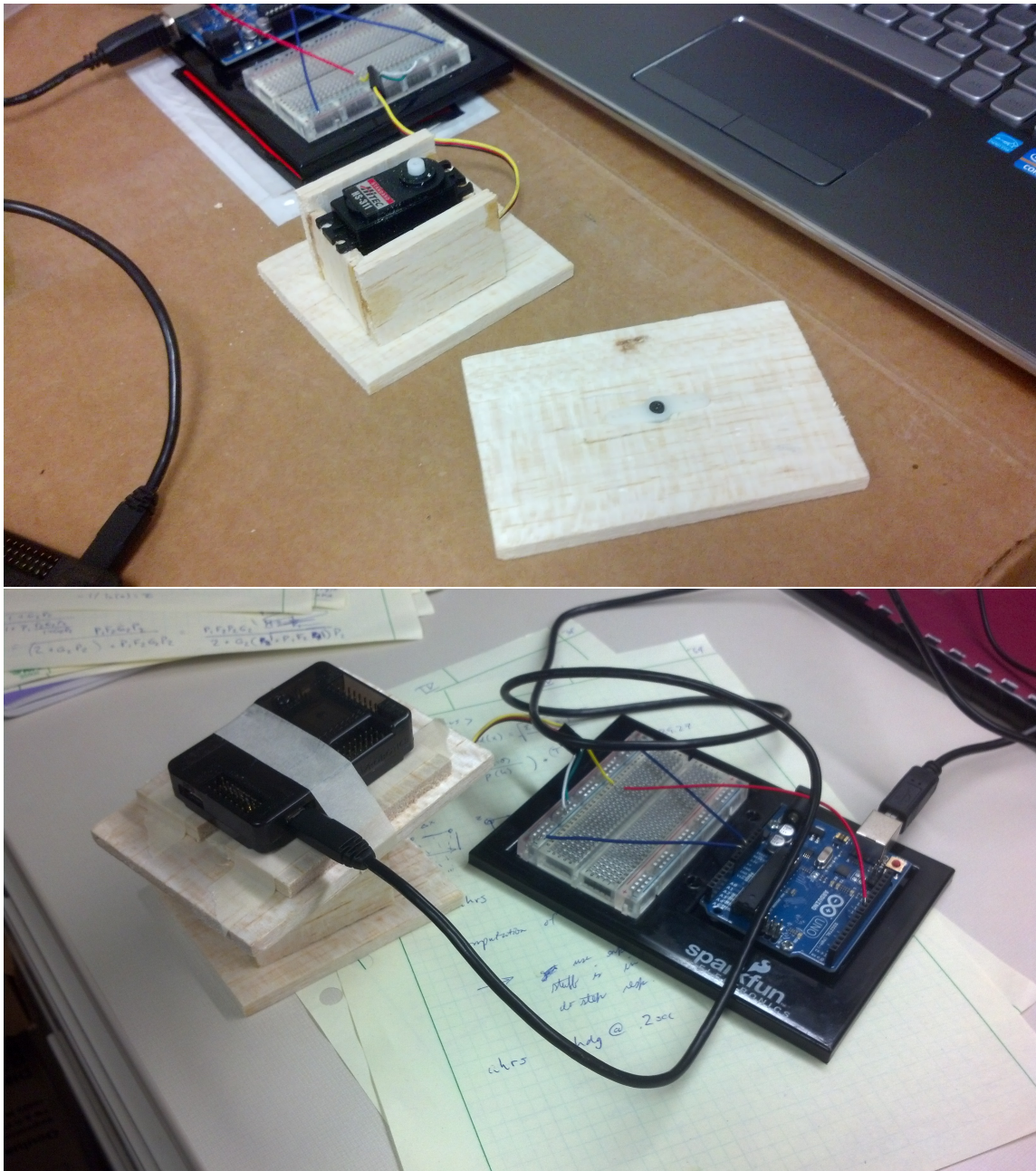
Figure 3.8: Test setup for APM2 AHRS error estimation.
