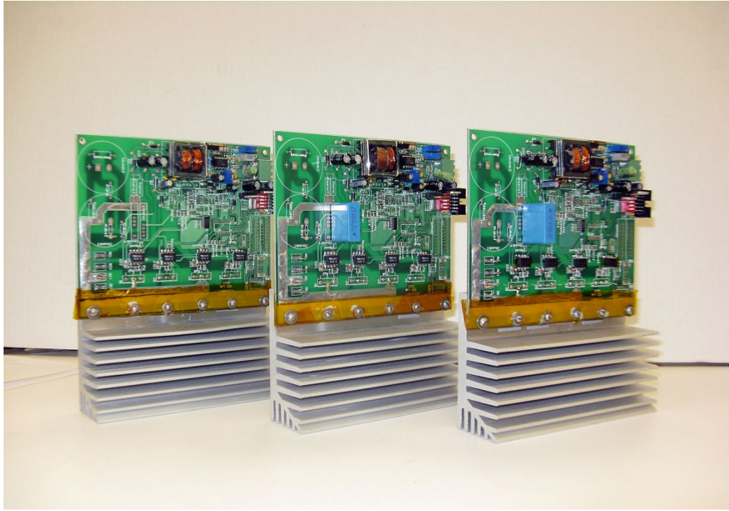
Fig. 3-4- H-bridges front view
