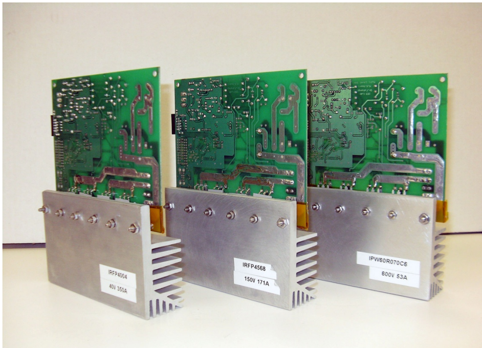
Fig. 3-5- H-bridges behind view
