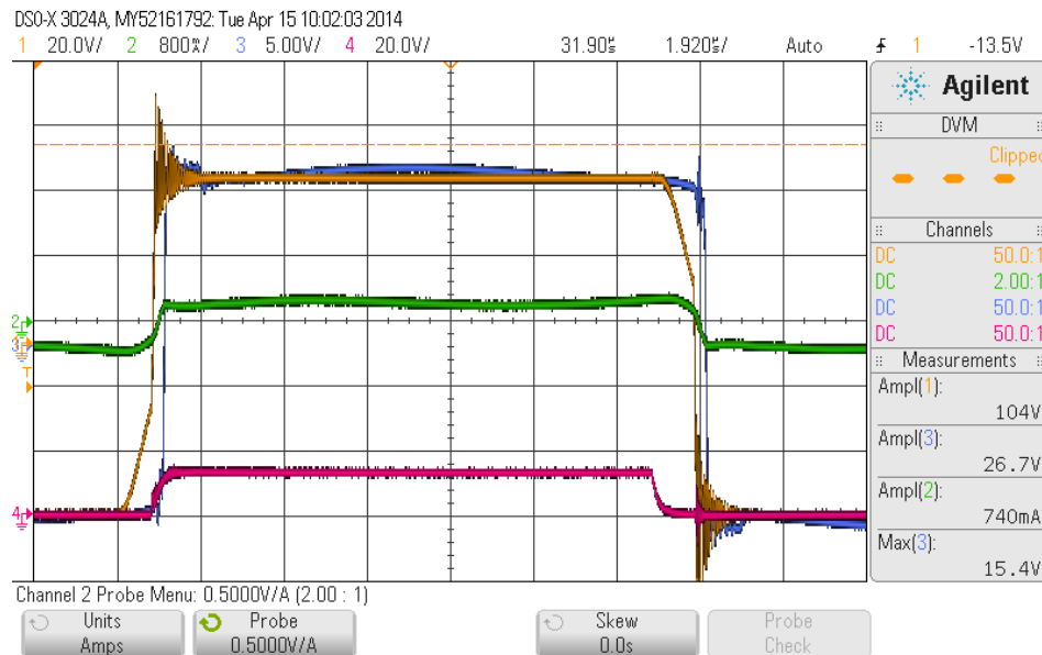
Fig. 6-3- DAB supplying R_L=25.1 \Omega , V_{in}=50.2 \text{ V} , \phi=15^\circ
