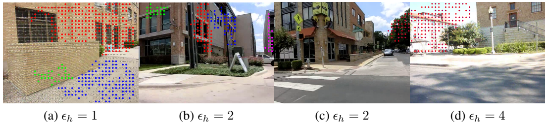
Figure 5.6: Example of extracted planes. Dots with different colors indicate different extracted planes. (a-b) show all planes extracted in the frame. (c-d) show two incorrect extractions.
