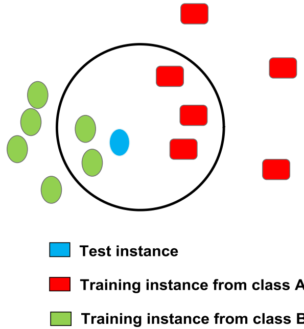
Figure 9. Weighted KNN classifier with K = 5 . The test instance most likely belongs to class B. But, it will be classified as A by majority voting. Distanced weighted KNN can avoid this by diminishing the vote value of instances from A compared to near placed training instances from B.
