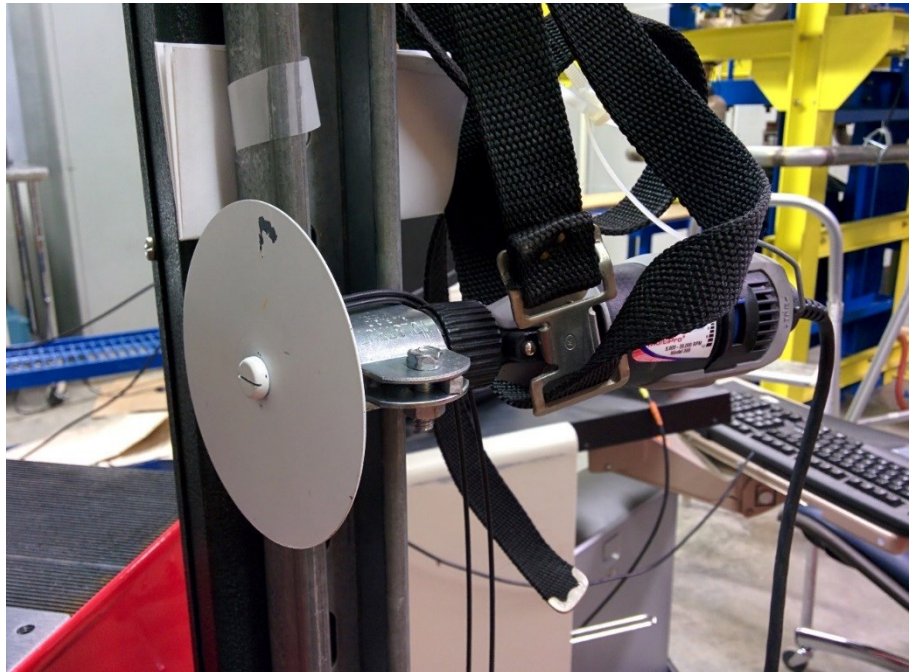
Figure 12 3.9 inch diameter rotating disc
