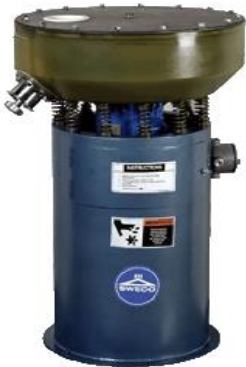
Fig. 5. Sweco DM1 vibro energy grinding mill used for the grindability studies.
