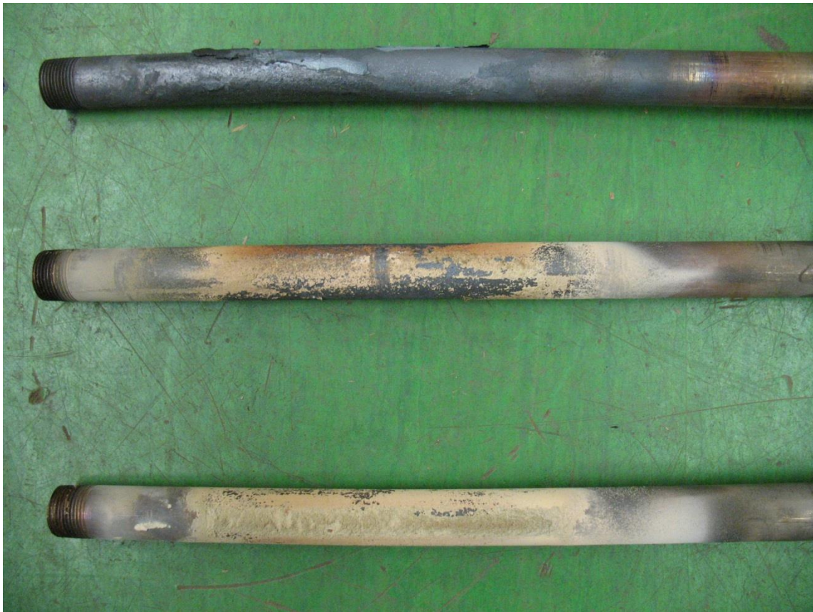
Fig. 59. Ash deposited on the surface of the heat exchanger tubes from the combustion of pure PRB; ER = 0.90.
