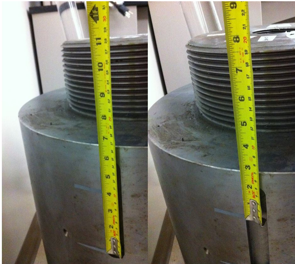
Figure B.14: Measurements of the keyholes used to verify with the -6dB method measurements (Testing I.3).
