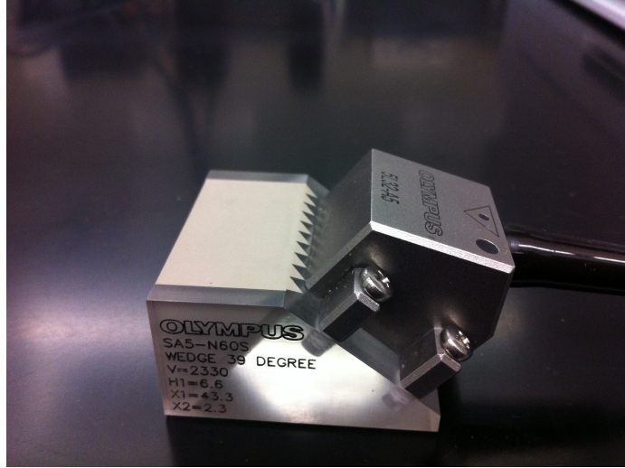
Figure 4.5: SA5-N60S 5L32 wedge and probe used for the exterior inspection of the grease hole.
