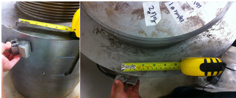
Figure B.2: Grease hole inspection of Hole #2 from the exterior curved surface (Testing E.2).
