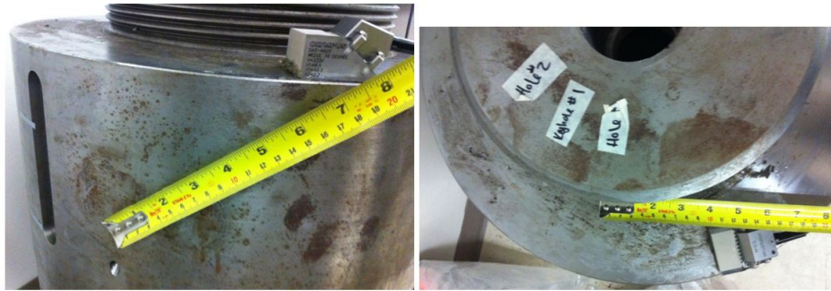
Figure B.1: Exterior scan of the grease hole from the top of the second level of the pin (Testing E.1).
