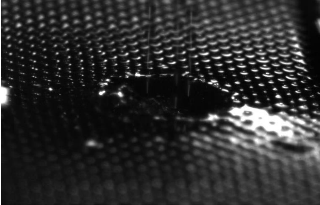
Figure 66. Triple stream droplets at 1000 \mu\text{m} spacing, with 100x100 copper mesh with 2.5 mm center hole with no heat flux
