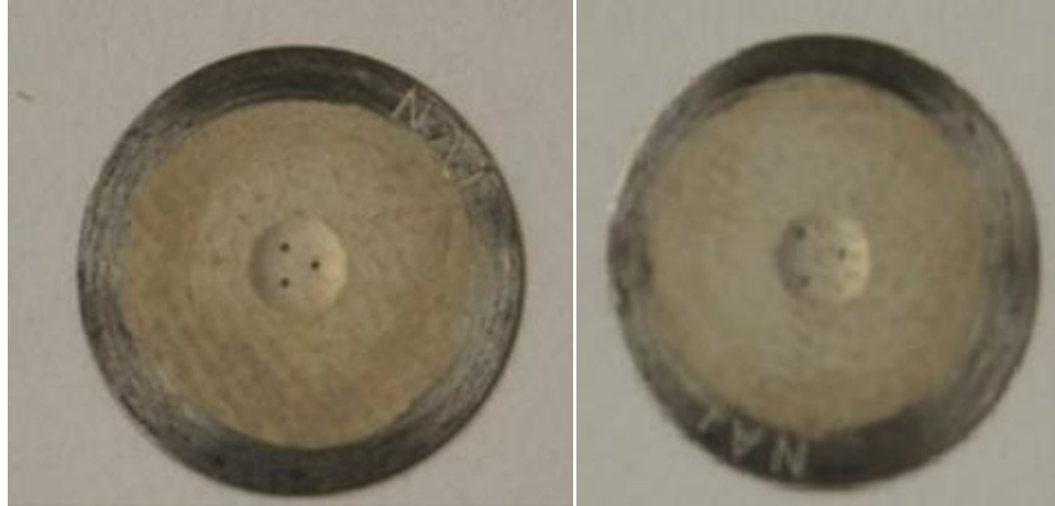
750 \mu\text{m} center to center orifice plate
