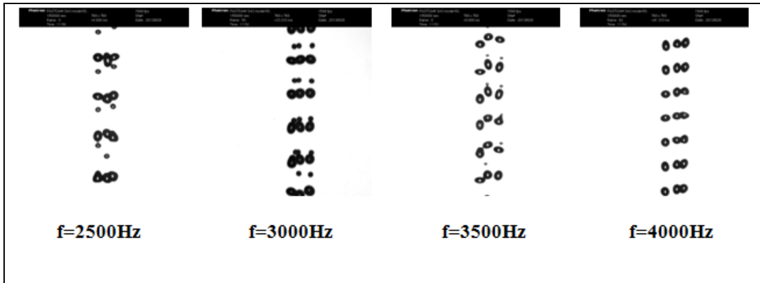
Figure 15. Image for multiple droplets with 750 \mu m center-to-center hole distance within the orifice plate at a flowrate of 450ml/hr.
