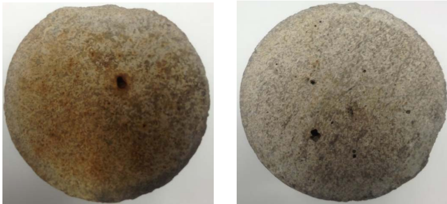
Fig. 4.20- Wormholes at the core inlet surface of the cores for an injection rate of (left) 2 \text{ cm}^3/\text{min} and (right) 10 \text{ cm}^3/\text{min} .
