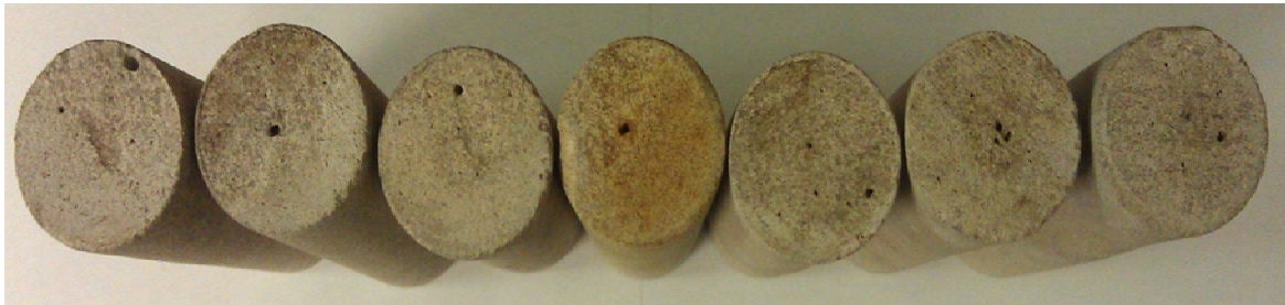
Fig. 4.18- Wormholes at the core inlet surfaces in order of increasing injection rate of 10 wt% sample D.
