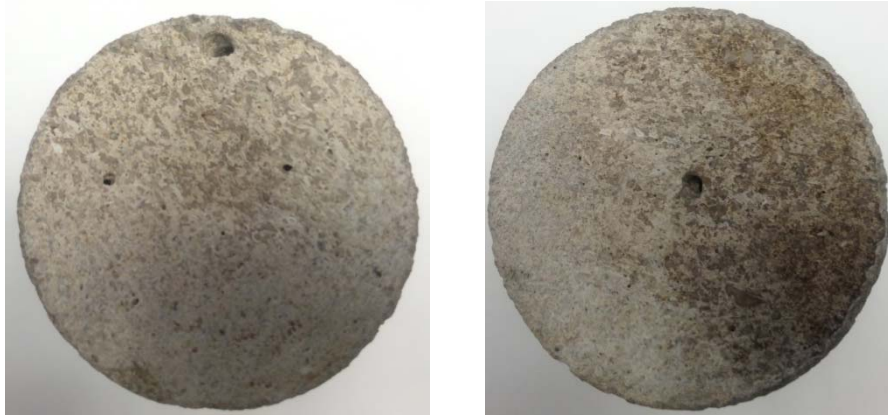
Fig. 4.19- Wormholes at the core inlet surfaces of the cores for injection rates of (left) 0.5 \text{ cm}^3/\text{min} and (right) 0.75 \text{ cm}^3/\text{min} .
