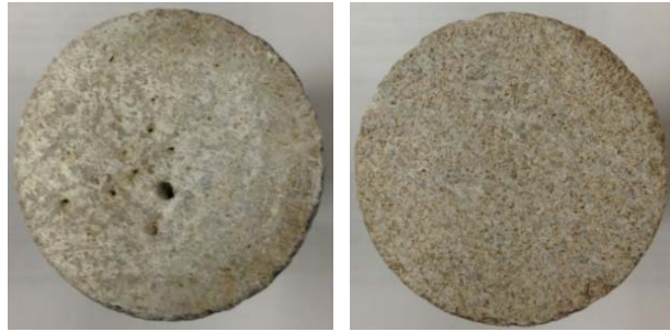
Fig. 4.3- Photographs of an Indiana limestone core used with sample A after treatment at 300°F (left) inlet face and (right) outlet face.
