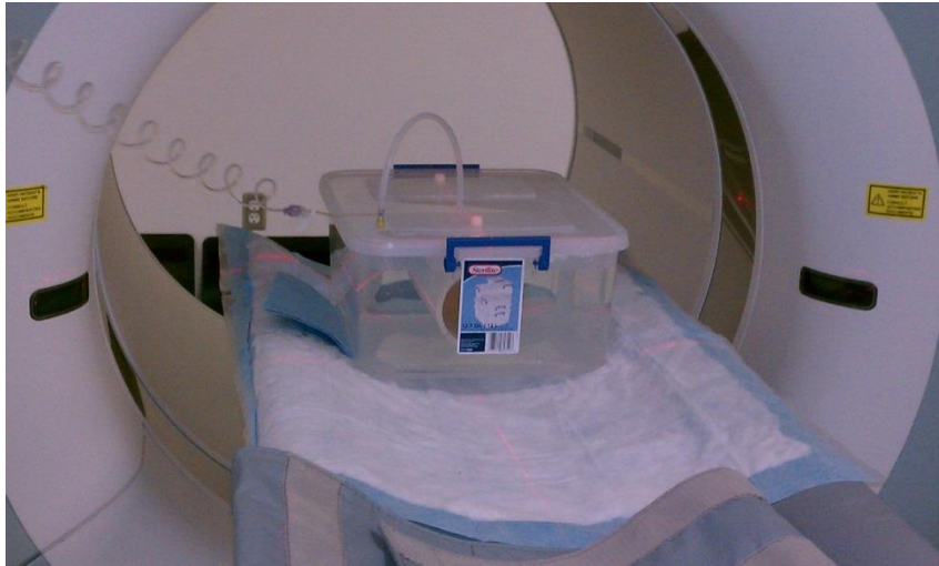
Figure 9. The phantom was scanning using CT.
