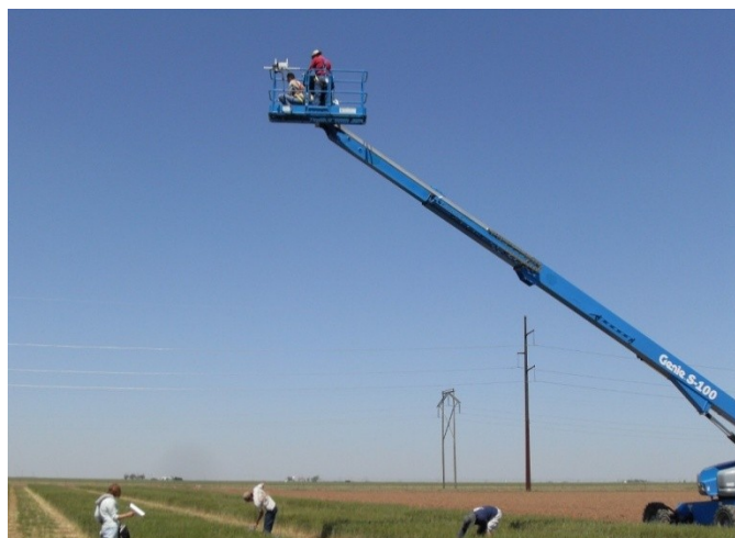
Figure 5.1. Thermal imaging of winter wheat plots using a boom-lift and on the ground using an infra-red thermometer in Bushland, TX in 2009.
