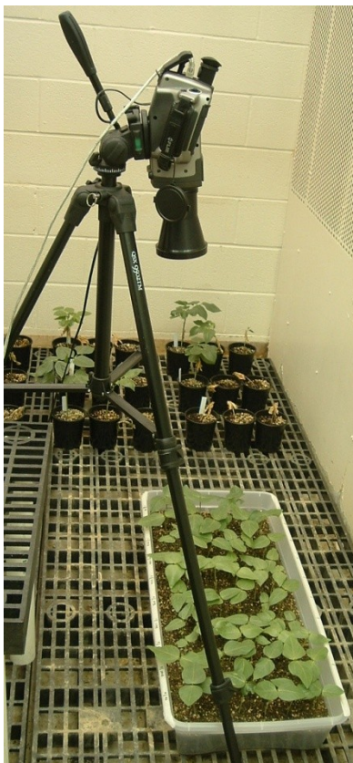
Figure E-1. Thermal camera on a tripod in a grown room configured to record thermal images of cowpea seedlings every 30 minutes 24 hours day -1 under drought box screening conditions.
