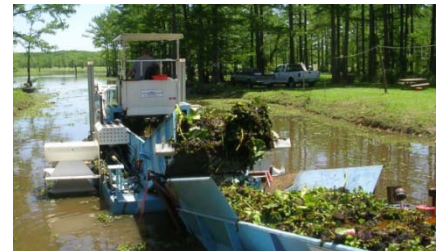
Mechanical harvester unloading harvested aquatic vegetation at Caddo Lake (photo courtesy of CLI)
