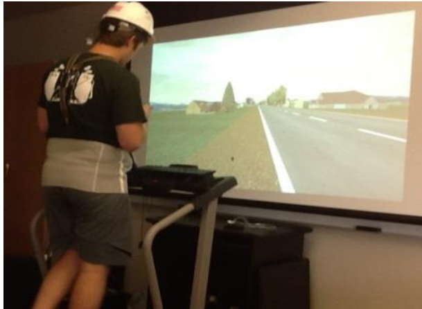
Figure 2. STISIM Drive ® driving simulator.
