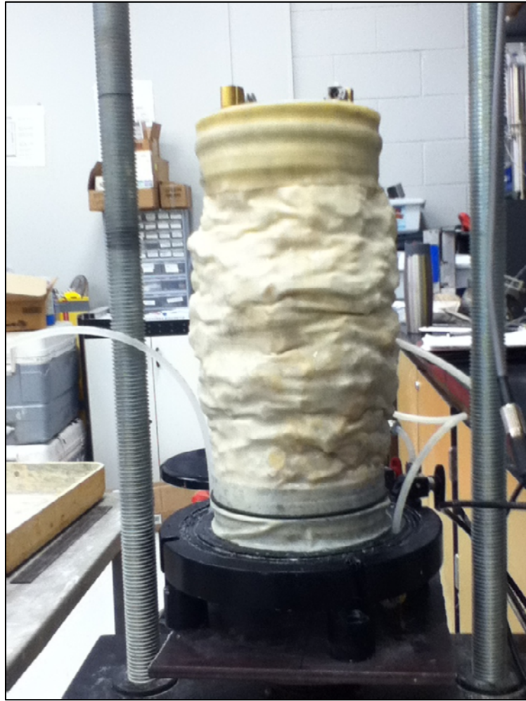
Figure 25. Parabolic Deformation of Test Specimen.
