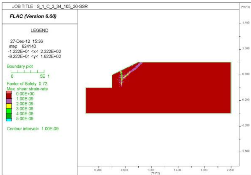
Figure B. 29. Series 1 Case 3 Foundation angle \phi=30^\circ , Backfill angle \phi=34^\circ and \gamma=105\text{pcf} Maximum Shear Strain Rate.
