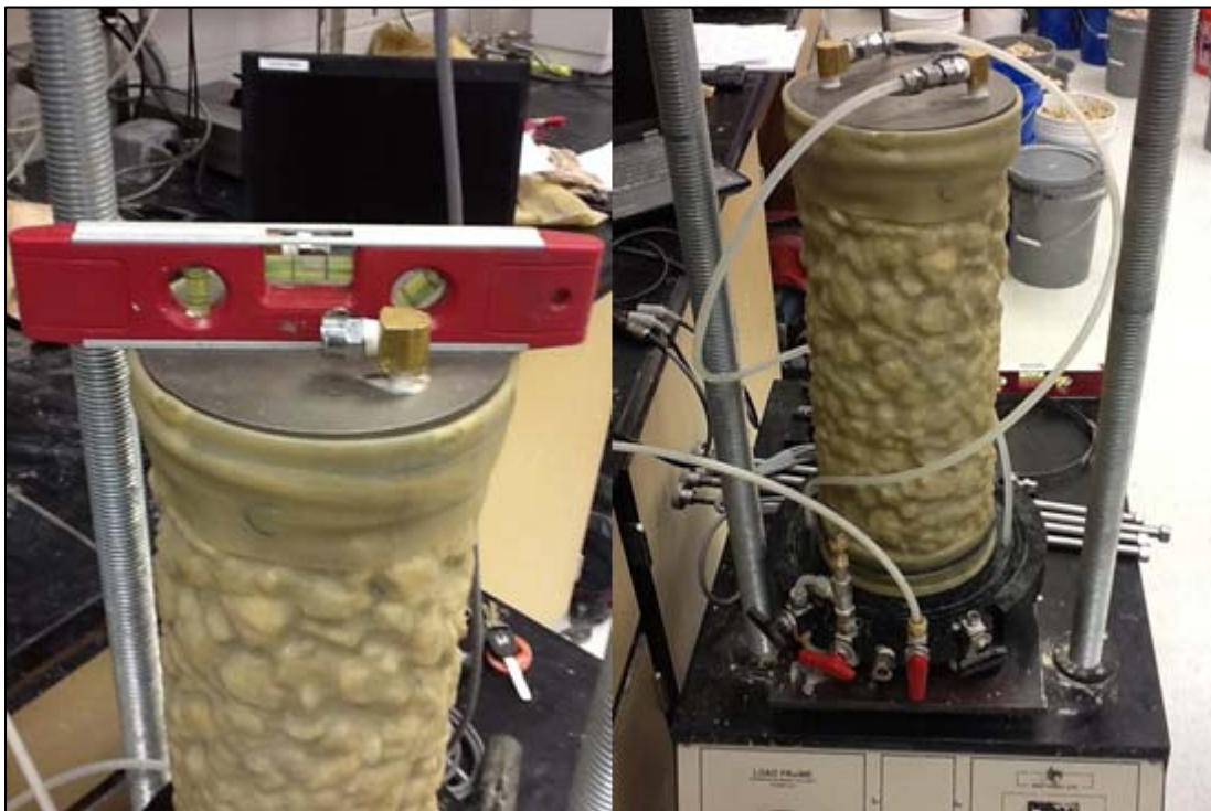
Figure 16. Leveling Top Cap of Specimen and Final Prepared Specimen.
