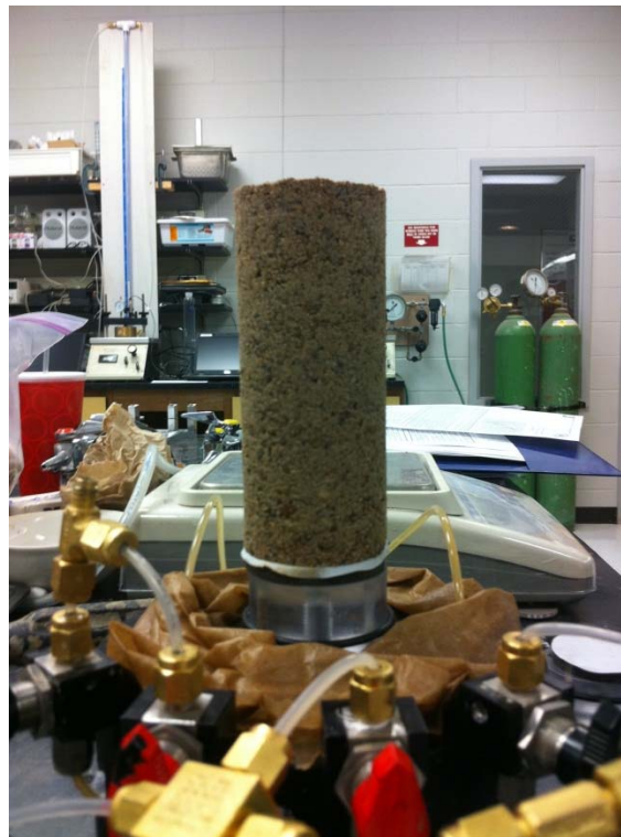
Figure 21. Sample Placed on the Bottom Cap of Triaxial Chamber.
