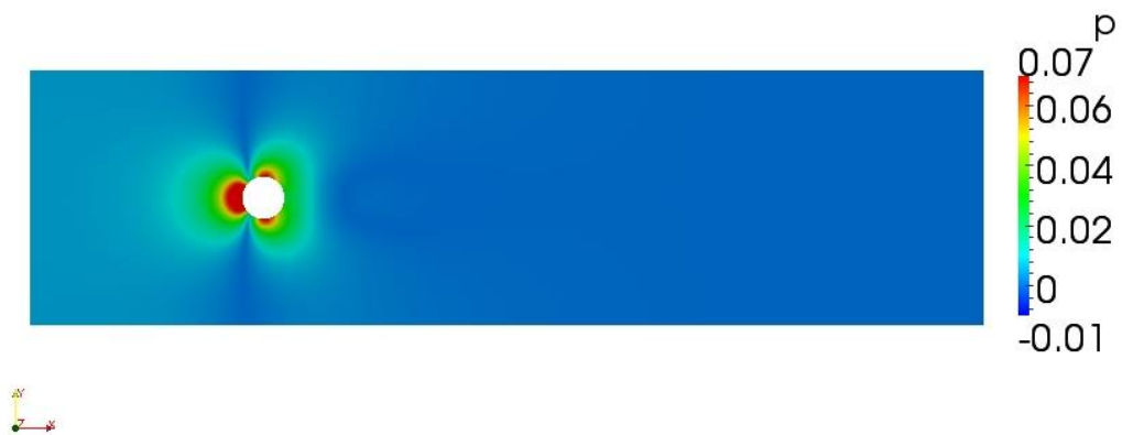
Figure 23 Pressure distribution of the flow past a sphere at Re=50
