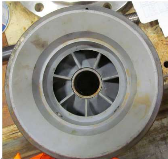
Figure 36. Diffuser Discharge View [24]
