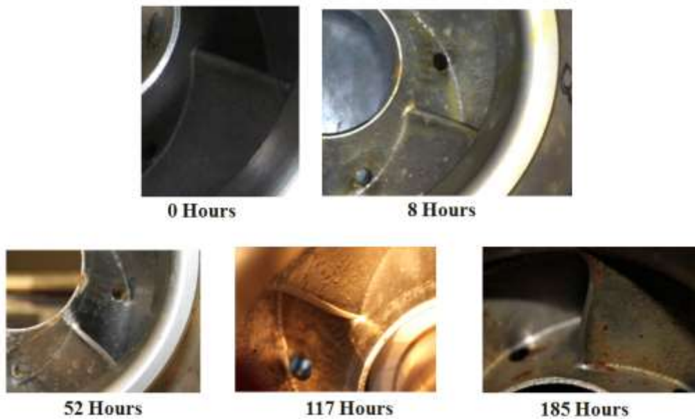
Figure 75. Wear Mark on Leading Edges
