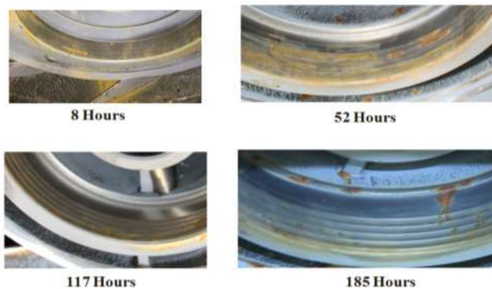
Figure 85. Contact Surface of Impeller Discharge Labyrinth
