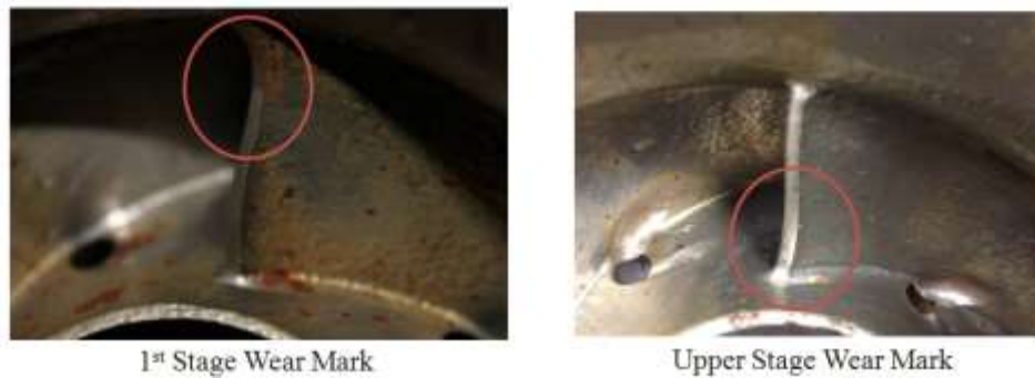
Figure 76. Wear Marks on Different Stages
