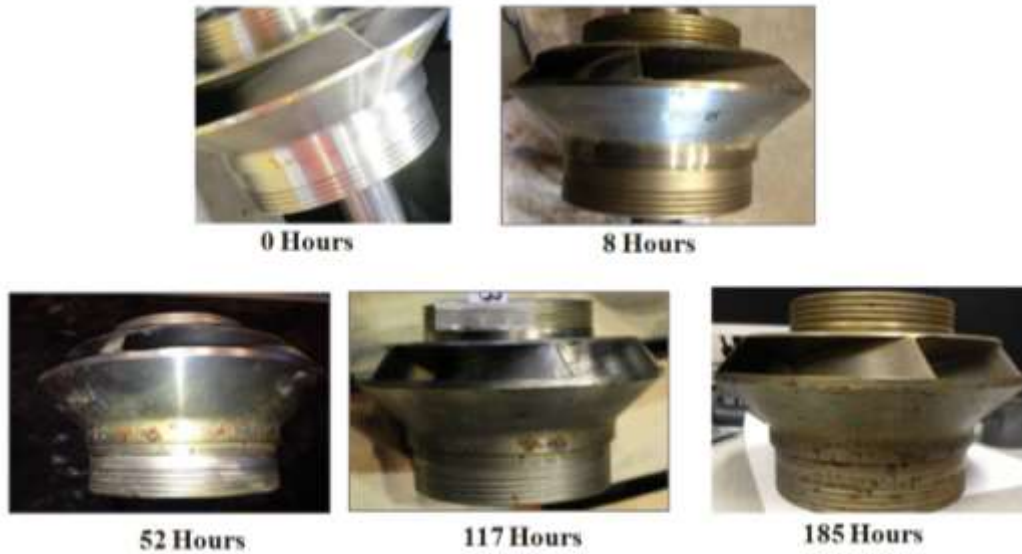
Figure 80. Wear Mark on Impeller Labyrinth Seal
