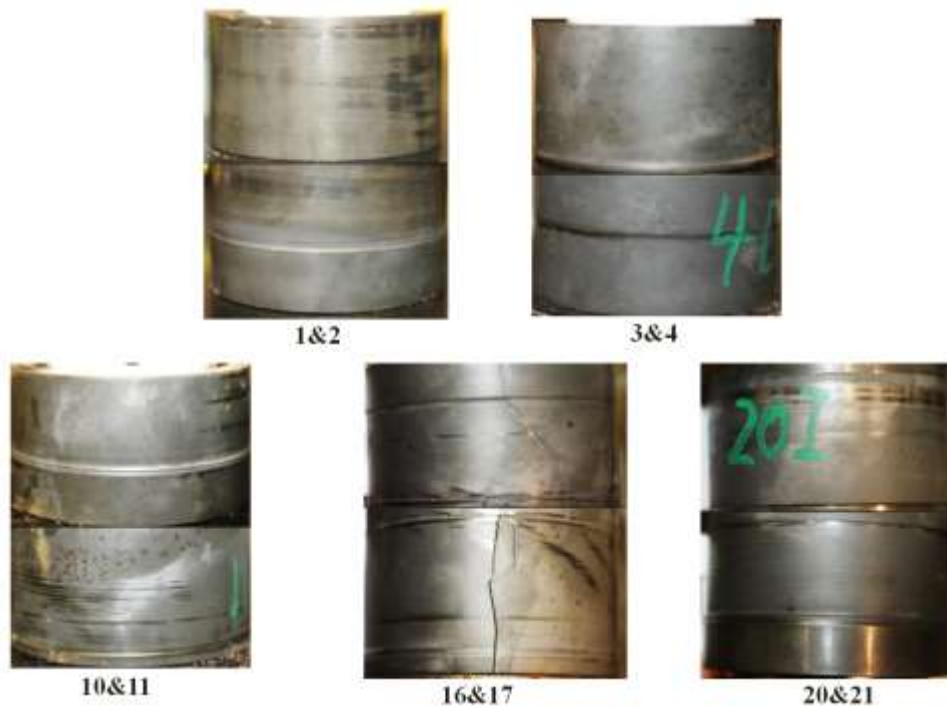
Figure 67. Bearing Status after Two-phase Test at 117 Hours
