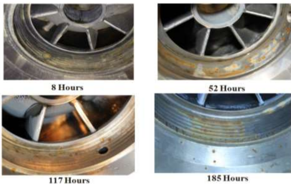
Figure 84. Contact Surface of Impeller Intake Labyrinth
