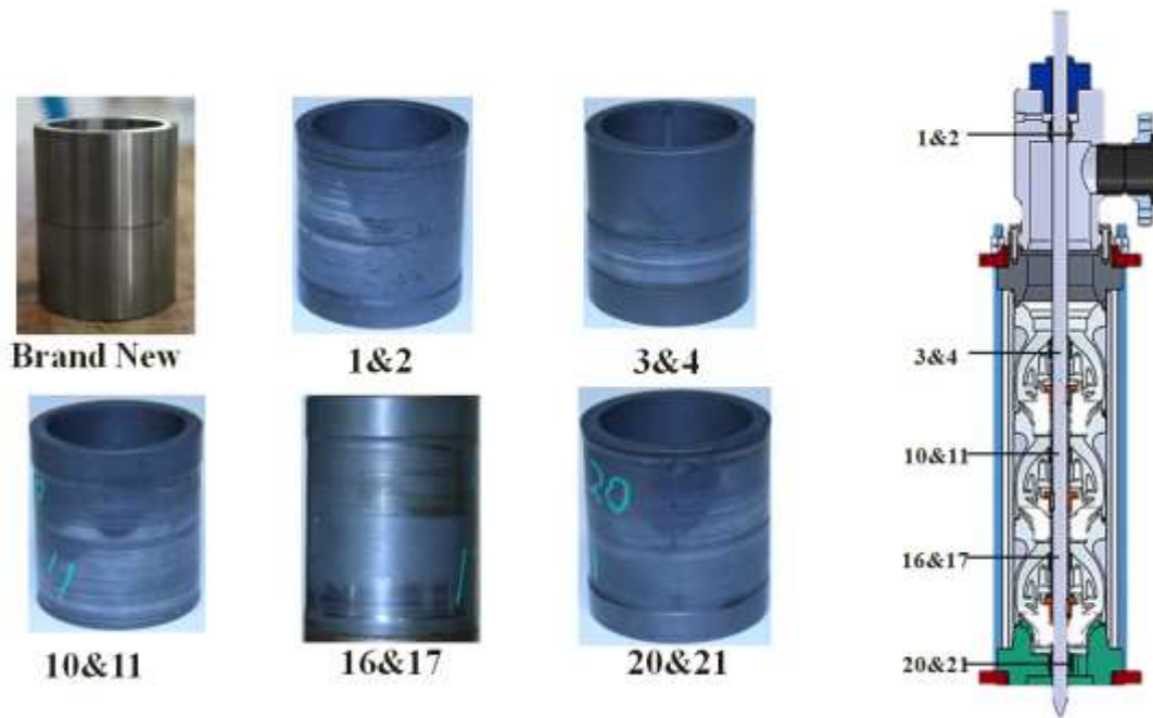
Figure 66. Journal Bearings Status after 185 Hours
