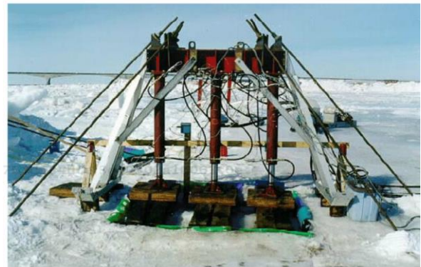
Punch shear test apparatus used in Canada in 1998 (KRCA)
