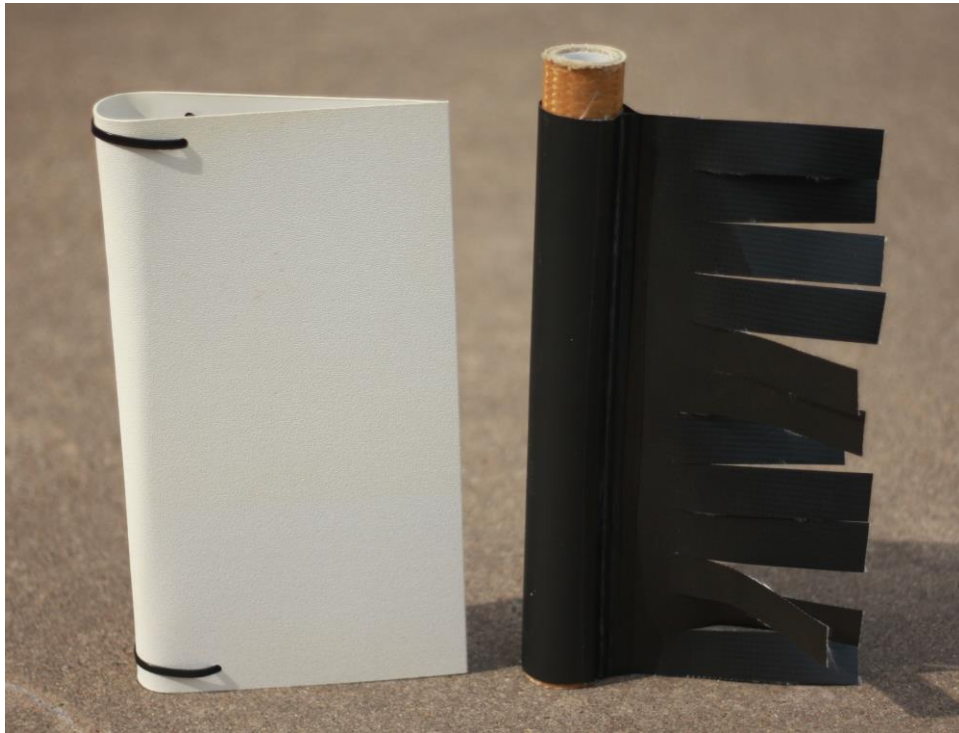
Fig. 3.2 Photographs of the airfoil (left) and ribbon (right) fairings used in the test.
