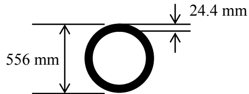
(b) Cross section of the pipe
