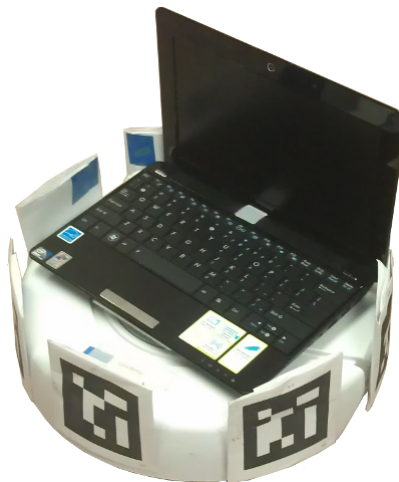
Figure 4.1: iRobot Create with mounted Eee PC netbook for webcam use. Markers placed around the robot are used by neighboring robots to determine relative position and orientation. © 2013 IEEE.
