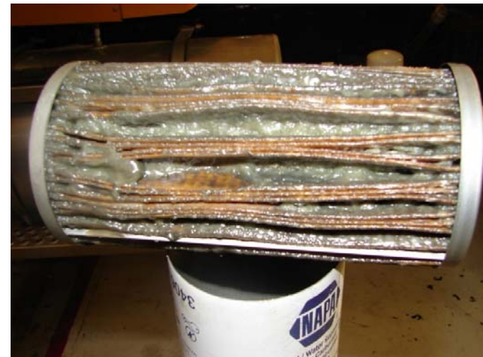
Truck Fuel Filter Biodiesel Gels in Cold Temperatures
