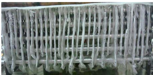
Figure 2. Evaporator with cotton wrapped around fins
