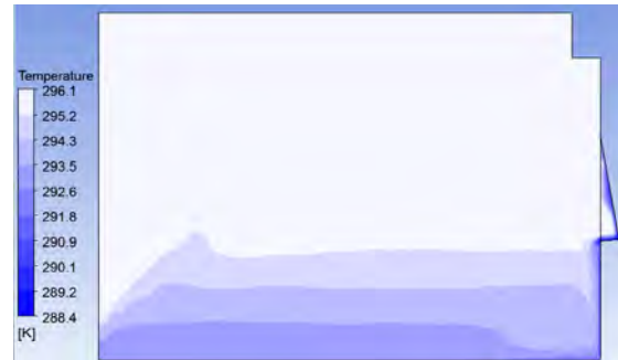
Figure 3.9. Air temperature distribution inside the room (plane through the middle of the door)
