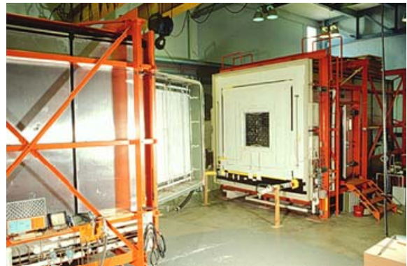
Figure 8 NRC-IRC guarded hot box
