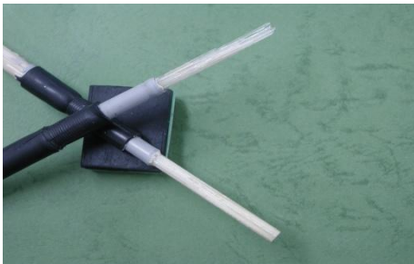
Fig. 9 Comparison of good and damaged cable ends (upper one is damaged)
