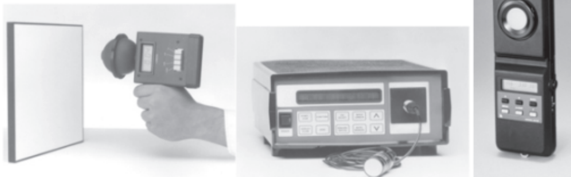
Figure 7: Commercial Illuminance Meters: (left) portable illuminance meter with integrating sphere, (middle) laboratory grade system that includes a photometer, radiometer and fiber-optic power meter, (right) multifunction portable illuminance meter with detachable receptor head.
