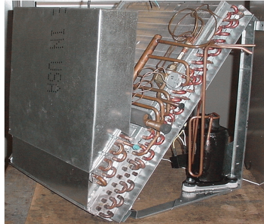
Figure 2. Air Handler with dehumidification system components
