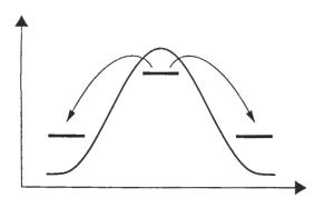
Figure 1 Thermal energy storage can "flatten" the utility load curve without eroding base kWh sales.
