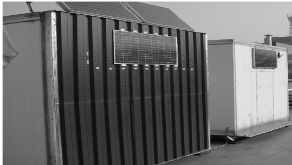
Fig. 3. Twin test rooms for PVT hybrid air heating system performance monitoring.
