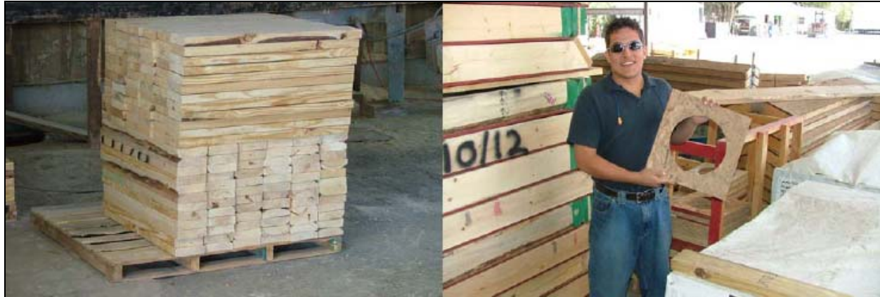
Figure 7. Reused dimensional lumber and OSB cut-off waste.
