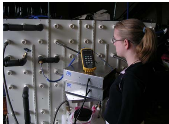
Figure 3. A middle school student operating a small-scale air conditioning system and gathering heat transfer rate data.
