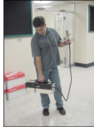
Figure 4. Tracer Gas Ventilation Rate Testing at a Florida School
