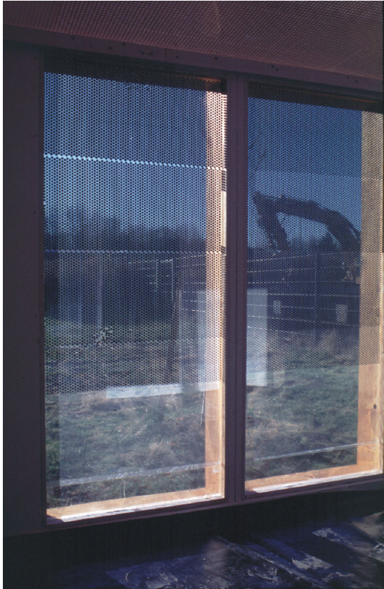
Figure 14 Testing glazings with different densities of ceramic frit
