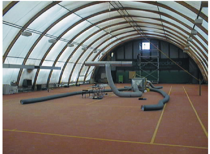
Figure 15 Measuring indoor air movements in an indoor tennis hall, experimental setting
