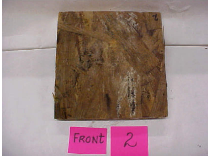
Figure 18: OSB with mold rating of 3
