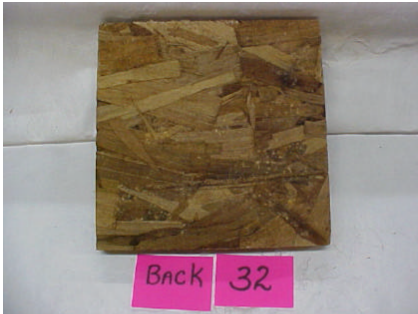
Figure 16: OSB with mold rating of 1
