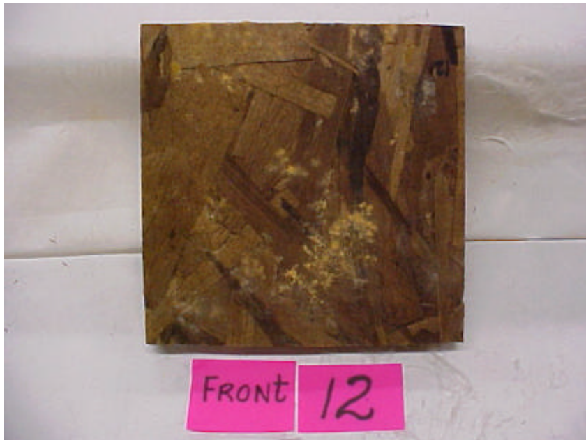
Figure 17: OSB with mold rating of 2
