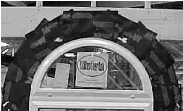
Figure 22: Self-adhesive modified asphalt flashing after thermal cycling (Wall C2)
