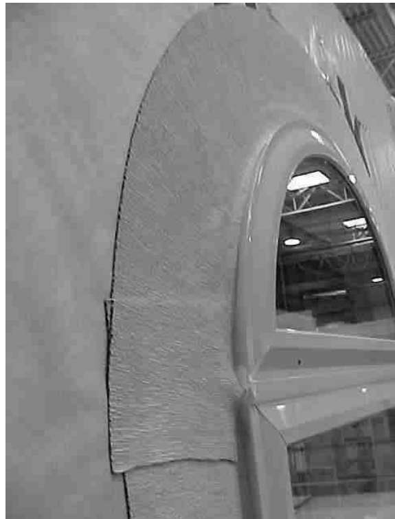
Figure 22: Self-adhesive modified asphalt flashing after thermal cycling (Wall C2)
