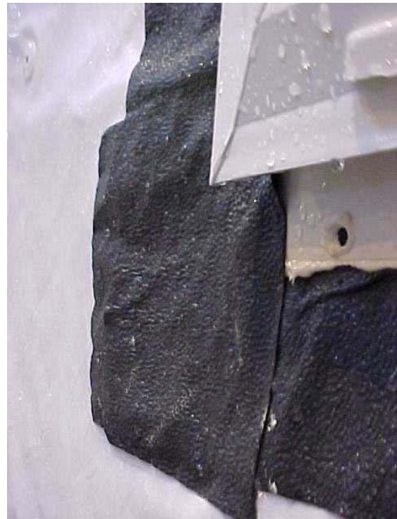
Figure 22: Self-adhesive modified asphalt flashing after thermal cycling (Wall C2)
