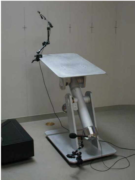
Figure 16: Representative heliodon, which allows table top movement below a fixed light source to simulate changes in latitude, time of year and time of day; building model would be placed on table top.
