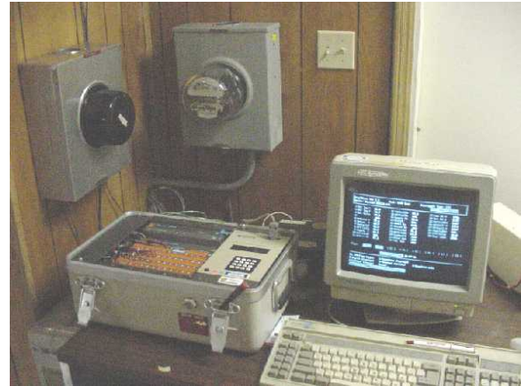
Figure 8. Data Acquisition Monitoring System for Side-by-Side Test
