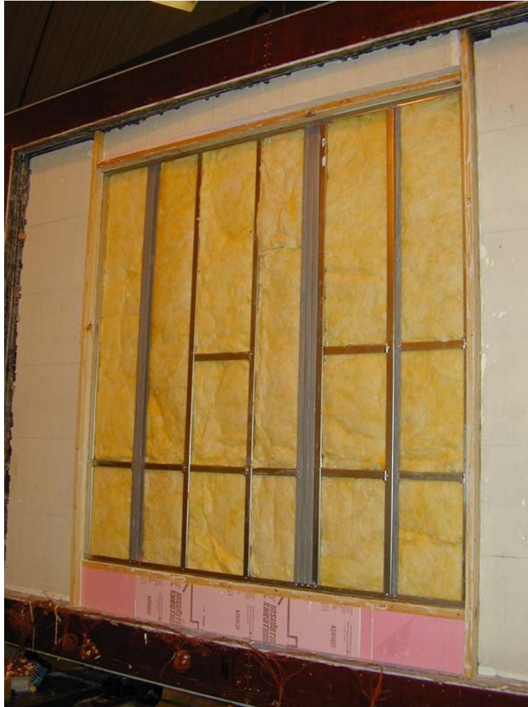
FIGURE 1. Steel Stud Wall Assembly with 24 % Framing Factor
