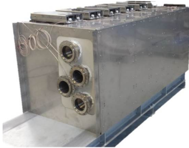
Figure 4.28: SOFC Stack Modules for the hybrid power plant at DLR. On the front side, the tubes that take the gas flows in and out of both anode and cathode can be noticed. On the bottom of the SOFC box, the sensors compartment is visible.
