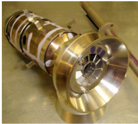
Figure 4.23: Burner with a single-can layout [50].
