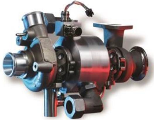
Figure 4.25: 3 kW Micro Gas Turbine studied at the Institute of Combustion Technology at DLR.
