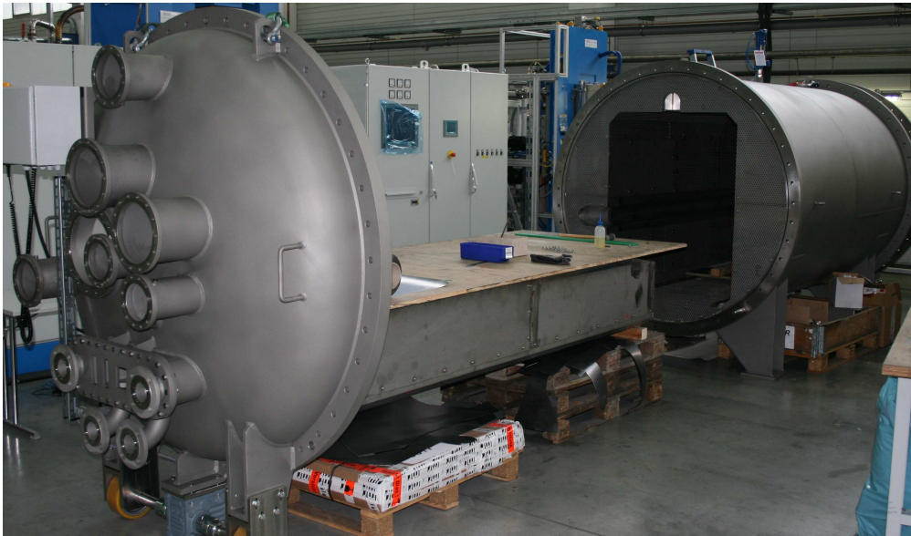
Figure 4.30: Open pressure vessel during fabrication.
